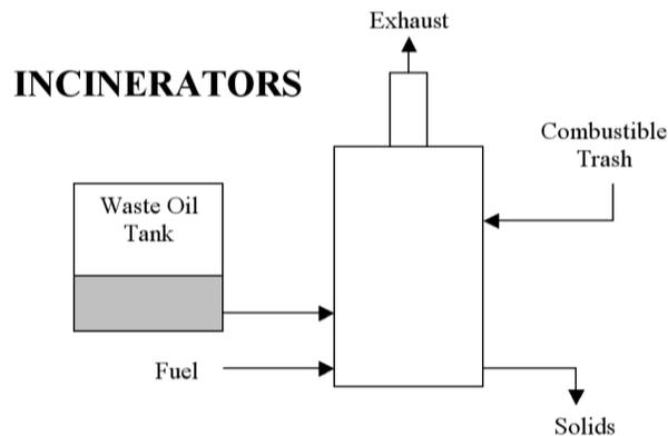
Shipboard incinerators are end stage devices that are used in various shipboard filtration systems, such as oily water separators and trash sorting systems. Incinerators can also be a component in ballast water treatment, closed loading systems and inert gas generators.
