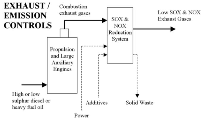
Most shipboard prime movers are diesel engines that burn the various grades of diesel fuel and heavy fuel oil. Diesel engines, especially highly efficient shipboard diesel engines that run on cheap high sulphur fuels, produce sulphur and nitrous oxides, which are considered to be major pollutants.
