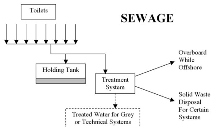
Just like in shore based sanitary systems, shipboard sanitary systems need a certain level of waste water treatment, which is controlled under MARPOL IMO regulations. On US flag ships sanitary treatment systems need to be United States Coast Guard approved, but USCG approval standards are identical to MARPOL standards. As such USCG approval can be obtained through certification by other national authorities.
