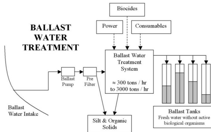
Most ships carry ballast and this ballast is generally in the form of water that is loaded in a cargo discharge port. While the cargo is being discharged the ship's pumps will take harbor water and load it into ballast tanks to ensure that the vessel floats sufficiently deep in the water to allow it to transit to another loading port. Once it arrives in the loading port it will discharge the ballast water into the loading harbor ecosystem while it takes on cargo.
