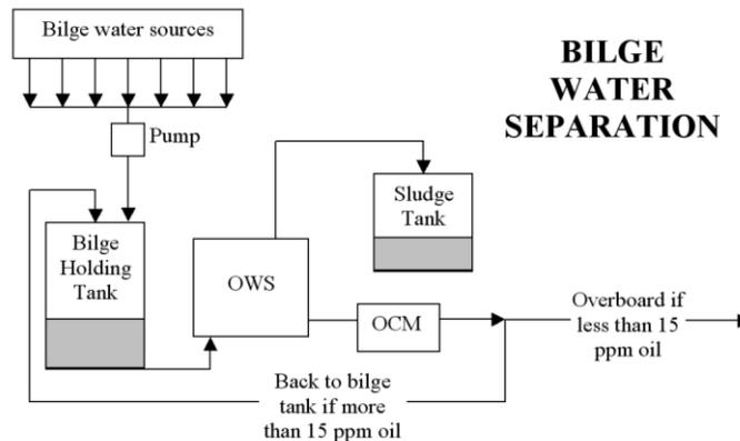
Bilge water is water that drains from shipboard systems and leaks into the lower portion of the ship (the bilges). This water is often oil contaminated and traditionally was simply pumped overboard when too much water collected in the bilges.
